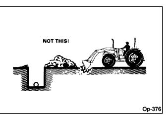
Leave dirt in bucket. Dumping on each pass wastes time.
